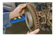
Remove the brake rotor. Follow the vehicle manufacturer's recommendations for rotor inspection and reuse.
