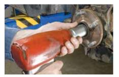
Remove the axle nut using an axle nut socket. Always refer to the vehicle manufacturer's instructions regarding nut replacement.
