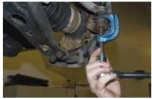
5. Remove the upper tie rod using the proper tool.
