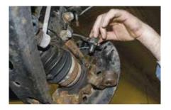
If present, disconnect the ABS sensor wire from its mating connector point and secure the sensor cable to prevent damage.
