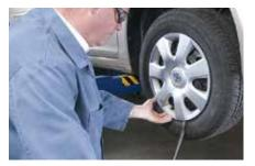
Raise the vehicle. Remove the wheel cover to access the lug nuts if needed. Remove the lug nuts and the wheel.
