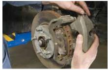
Remove the caliper and the caliper mounting bracket. Make sure to properly support the caliper with either an "S" hook or a piece of wire to prevent brake line damage.
