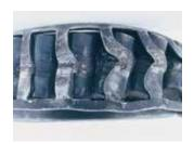
**Total bearing lock-up:** Rollers skew and slide sideways.
