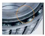
Bearing cone (inner race) large rib face deformation: Metal flow from excessive heat generation.
