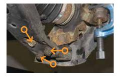
4. Install the bolts that attach the lower ball joint to the lower control arm. Torque the bolts to the vehicle manufacturer's specifications.
