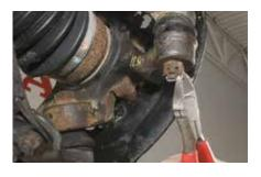
6. Secure the nut using a new cotter pin.
