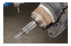
Inspect the surface of the axle shaft, spline teeth and tone wheel for wear. Use a fine file, wire brush, emery cloth or honing stone to remove any debris, nicks or burrs.
