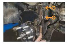
Install the strut mounting bolts that attach the steering knuckle to the strut assembly.
