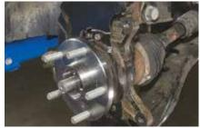
To prevent spline damage, check the position of the splines while installing the steering knuckle. Never force the hub unit bearing assembly onto the shaft or strike with a hammer.
