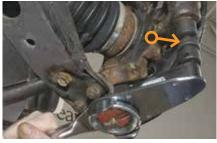
5. Attach the lower ball joint to the lower control arm and install the nut. Torque the bolts to the vehicle manufacturer's specifications.
