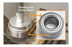
2. Press the new bearing into the steering knuckle using an appropriate press and support fixture. The outside diameter of the tooling surface must be large enough to support the bearing cup (outer race) of the bearing assembly.
