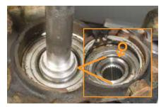
2. Remove the hub stud from the bearing, using an appropriate press and support fixture.
