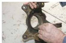
Clean the steering knuckle of debris or burrs using a fine file, wire brush, emery cloth or honing stone.
