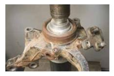
Remove the bearing from the steering knuckle using an appropriate press and support fixture.
