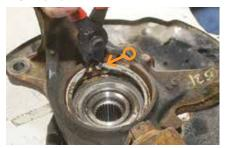
Remove the bearing retaining snap ring from the steering knuckle using a pair of snap ring pliers.
