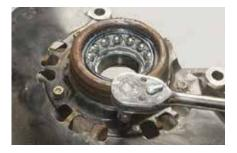
3. Remove the disk brake dust cover.
