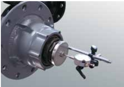
Fig. 3 – A typical end play gauge.
