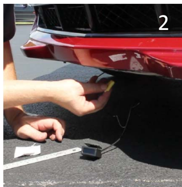
2 Wipe 3M promoter for sensor & wire clips mount.
