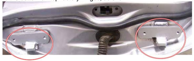
6) Installing the hinge to the door.
