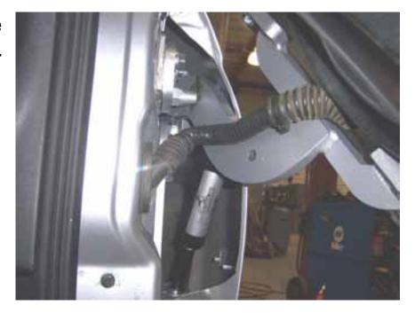
**14)** Cut the inner lip of your fender to make room for the new Vertical Doors hinge. Note: After you have cut the fender use a sander or grinder and make sure the surface is completely flat.
