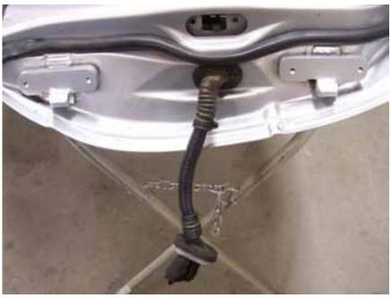
wire slack use the clips or zip ties to secure the wires. You will have to cut the factory wire loom in half, later we'll add wire loom to protect the exposed wires.
