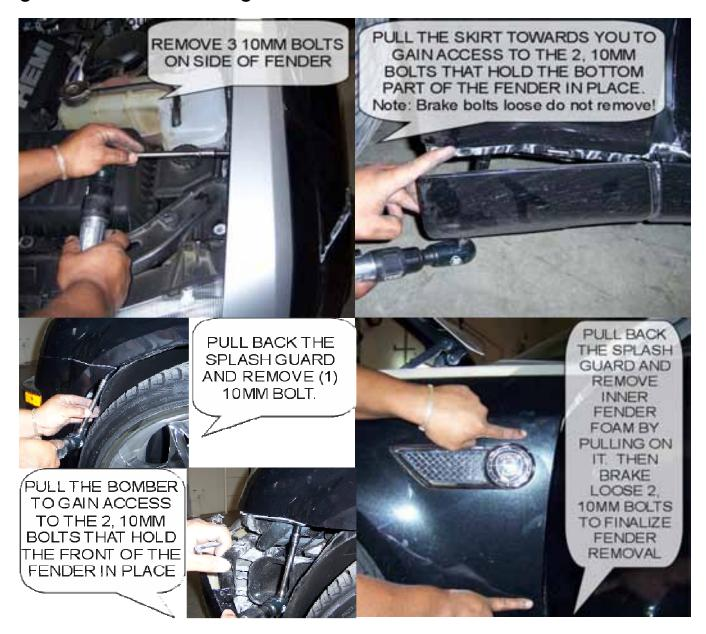
To remove the fender lift up the top of the fender toward you and then slip out the bottom end. 3) Modify the spot where the New Vertical Doors hinge will be located. Note: surface must be completely flat before installing the New Vertical Doors hinge.
