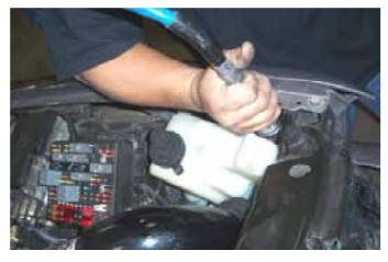
Remove one 13mm bolt from the bottom of the door securing the fender to the chassis.
