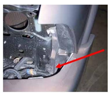
Remove all the 13mm bolts from the top of the fender and one bolt from the front of the fender by the headlights.
