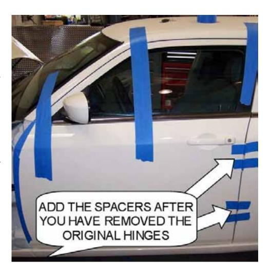
6) Remove original door hinges and Install the New Vertical Doors Inc. System.
