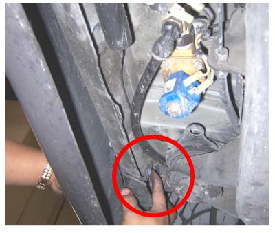
Remove all the 12mm bolts and the 13mm bolts from the wheel well.
