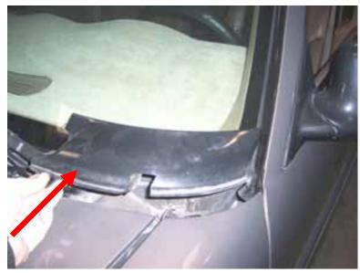
After removing the cover you will be able to remove the last 13mm bolt on the hood hinge.
