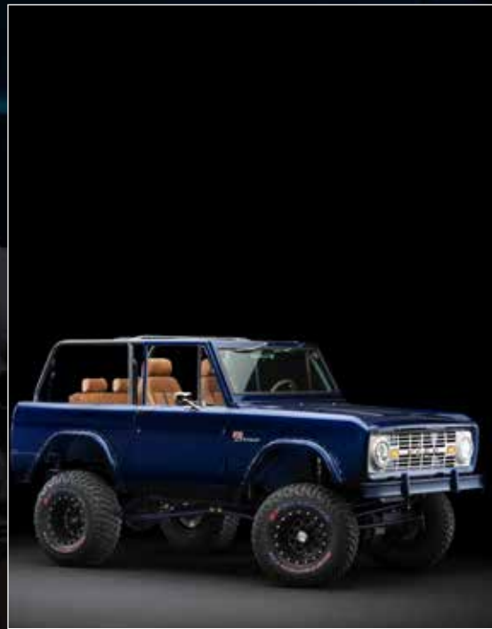
United Pacific partnered with Maxluder Brothers for the 2018 SEMA Show, to build this custom '74 Ford Bronco using our steel replacement panels and LED lighting.
