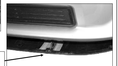
Hold the splash guard up to the brackets and mark location for cutting to clear brackets. Cut only what is needed to insert bracket through the splash guard.
