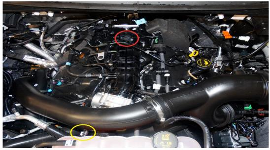
2. Now you will want to locate the Turbo Charger Pressure Sensor and the MAP Sensor both shown on this picture. The Turbo Charger Pressure sensor is identified with the yellow circle while the MAP sensor is identified with the red circle.
