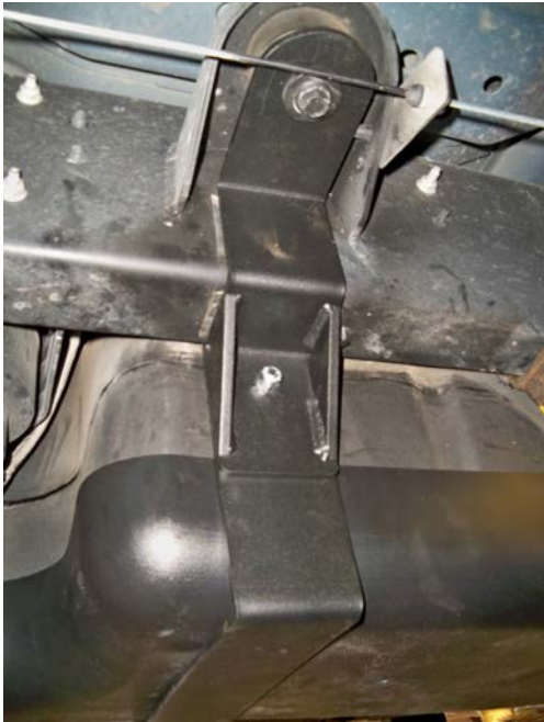
(Fig. 14) Completed front support installation on tank with TITAN Shield.
