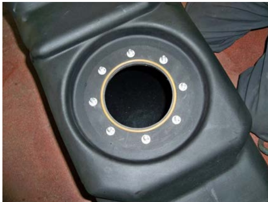
(Fig. 3) Leave the “O” ring gasket, studs and retainers assembled as they are (shown before sending unit, top flange, and 5/16” nylon locking nuts are installed).
