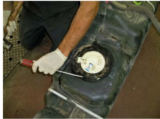
(Fig. 2) Loosen hold-down ring on original equipment tank by tapping counter-clockwise, remove and lift out sending unit.
