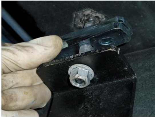
(Fig. 8) Thread two shims onto each strap bolt.
