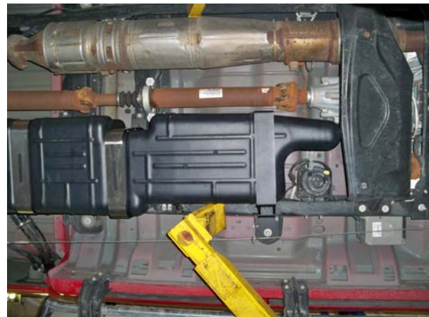
Underside view of TITAN 2011 Crew Cab Long Bed tank (7020311) with shield installed in an F450.
