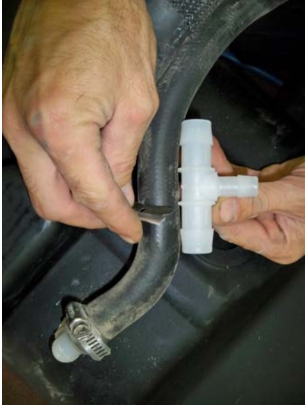
(Fig. 6) Cut \frac{3}{4} " vent line hose approximately 4 \frac{1}{2} inches from elbow end of hose.
