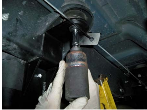
(Fig. 13) Replace cab mount bolt with its existing washers and tighten to factory specification.
