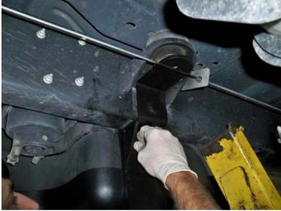
(Fig. 12) Mount the upper piece of the assembly to the lower piece using bolt provided.
