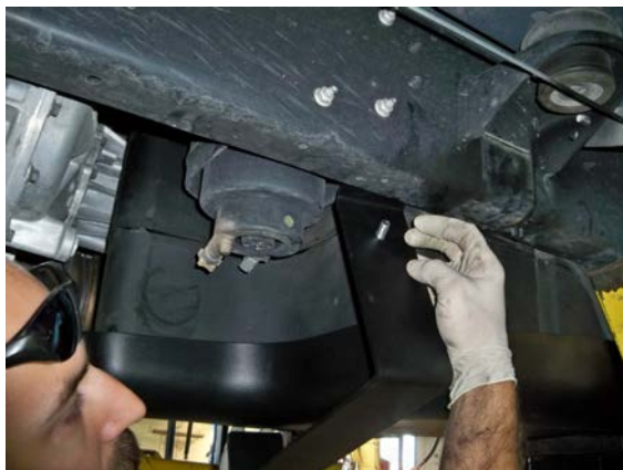
(Fig. 10) Hang lower piece of support assembly on lower lip of vehicle frame and slide towards the rear of vehicle until it lines up with cab mount.
