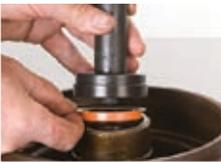
The grease seal must be replaced when it leaks or when bearings are being repacked
