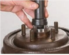
Use a cup driver or mild steel bar to press or drive the new inner cup and outer cup into the
