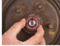
Slide the rotor/hub assembly back over the spindle, being careful not to damage the
