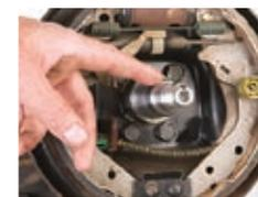
clean the rotor/hub assembly and spindle with kerosene or mineral oil. In-
