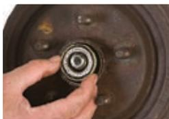
Follow the vehicle manufacturer's recommended procedure to remove the tire and wheel assembly, disk brake caliper, dust cap, cotter pin, adjusting nut and washers.
