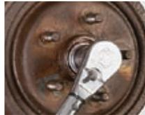
Use a torque wrench to tighten the adjusting nut to 50 ft. lbs. while turning the rotor. Back
