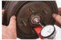
Use a dial indicator to measure end play. Mount the indicator base as close to
