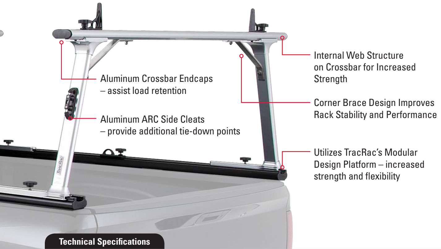
Sliding Racks Adjust Along Full Length of Bed to Carry Different Loads and Can Easily Be Removed When Needed
