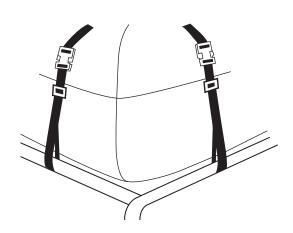
This product requires a roof rack in order to attach to vehicle. Included compression straps attach to raised side rails, to raised cross bars or to both.
