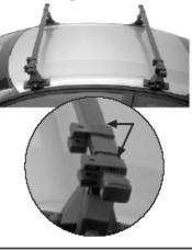
Loosen nuts to adjust rear bracket
