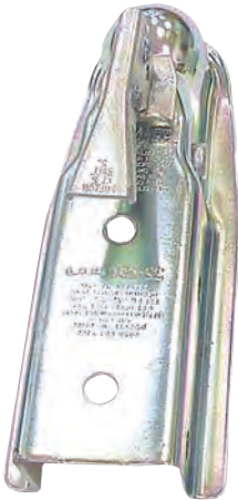
Fulton coupler after 336 hours salt spray testing.
