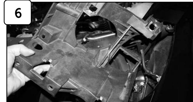
Carefully pull all harness away from bracket and remove.
