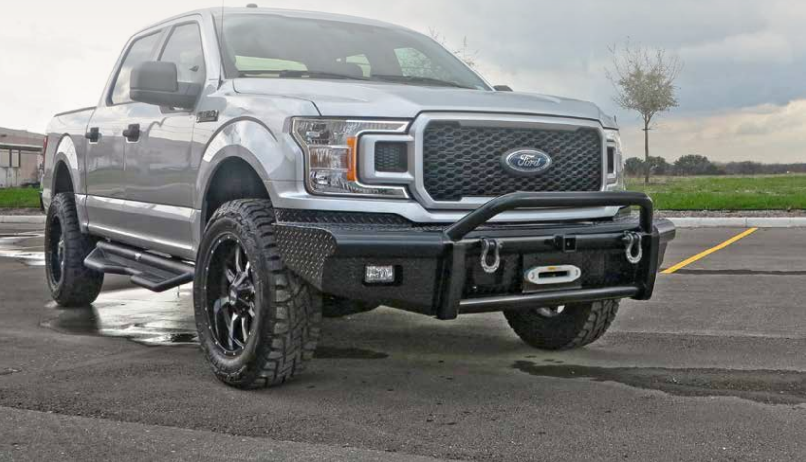
Convenient removable panel for easy winch access
