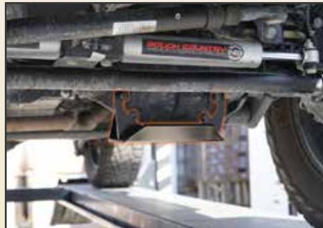
Differential protection with drain plug cutout
