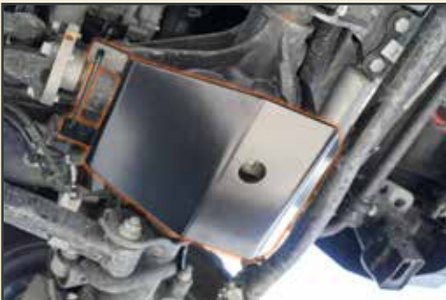
Differential protection with drain plug cutout
