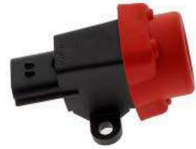
FV-7 Fuel Pump Cut-Off Switch 88922295
