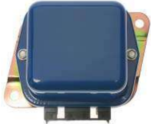
VR-613 Voltage Regulator J8130365; J8130365; J8130365; J8130365; J3227716; J3227716; J3227716; J3227716; D7PF10316AA; D2TZ10316AA; D3AF10316AA; D3TF10316AA; D4AF10316AA; D4TF10316AA; C5AZ10316A; C5TF10316A; C8AF10316A; D0AF10316A; D2TF10316AA; C3XF10316C; C4SZ10316A; C4UF10316A; C4UF10316B; C5AF10316A; F0PZ10316A; C3SZ10316A; 1972270; 12322746 American Motors ..... 1979 - 1976 DeTomaso ..... 1974 - 1971 Ford ..... 1985 - 1965 Jeep ..... 1977 - 1976 Lincoln ..... 1978 - 1963 Mercury ..... 1978 - 1963
