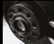
2 Wheel hub with disassembled grease cap
