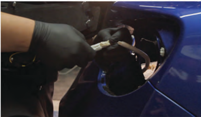
7) Connect the Spyder tail light to the wiring harness.
