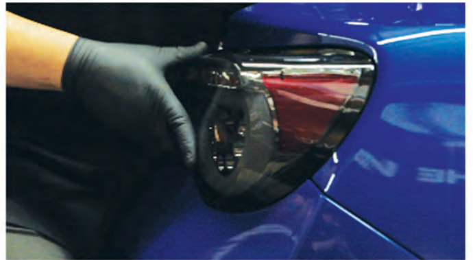
8) Seat the Spyder tail light, taking care not to pinch the harness between the tail light and body.
