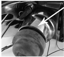
To avoid condensation, make sure the rubber seal is on tightly. If not, moisture will build up.
