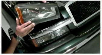
2) Unseat the headlight and disconnect the headlight wiring harnesses.
