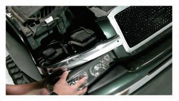
5) Reinstall the DRL socket and turn signal socket into the SPYDER lower lens assembly, then seat the lower lens assembly.
