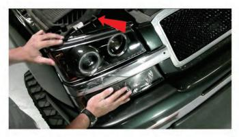
7) Reinstall the headlight retainer stake to secure the upper headlight lens assembly.
