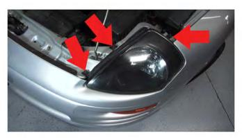
1) Open your hood to reveal the headlight assembly. In order to unmount the headlight you will need to remove (3) 10mm bolts that hold the headlight in place. The locations are indicated by the red arrows.
