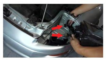
2) Once the bolts have been removed, you will need to remove the headlight harness connected to the OEM headlamp, shown here. Once the harness is disconnected, pry the light assembly free.
