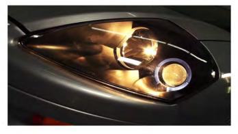
4) Lastly, test the new headlight assembly. Low beam and high beam will only come on individually and will not stay on together. Above is for reference only. Halo LED's require additional wiring;
