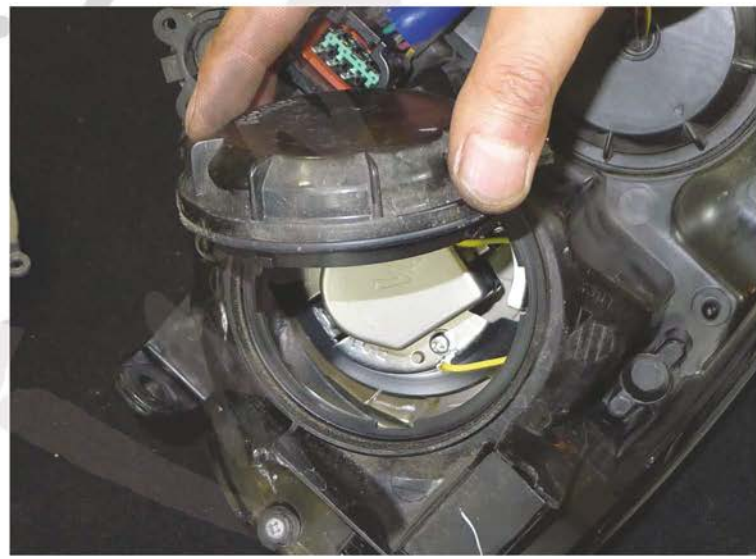
26. Remove the light bulb access hole cover
