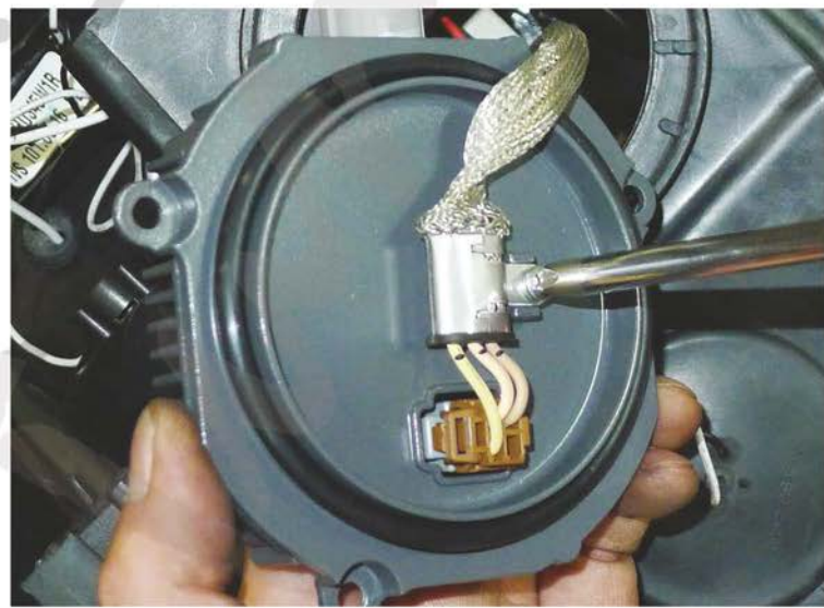
38. Secure with the phillips head screw
