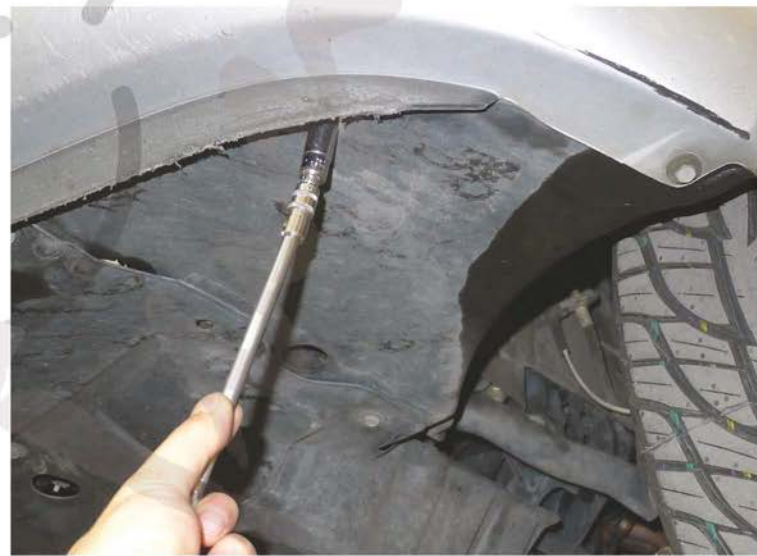
50. Tighten the (10) 10mm bolts. Please repeat the steps from 1 to 50 for the opposite side
