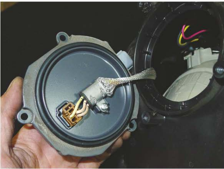
23. Back of the ballast
