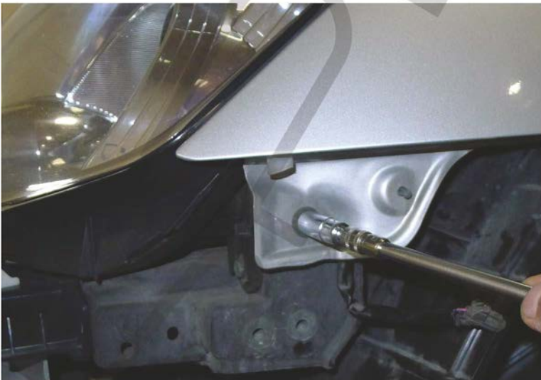
15. Remove the 10mm bolt
