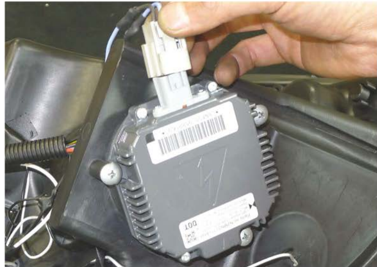
40. Connect the headlight harness to the ballast
