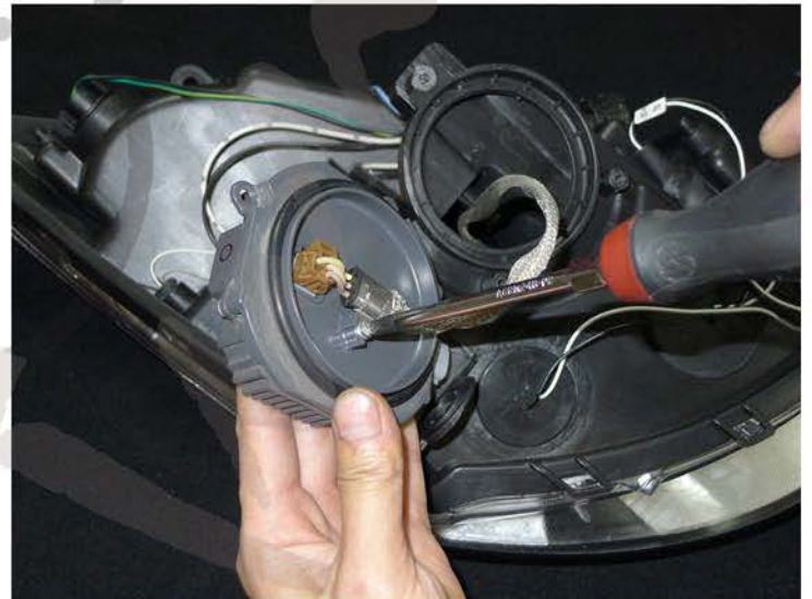
32. Tighten the phillps head screw
