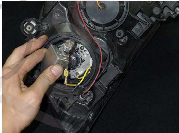
26. Disconnect the HID light socket and remove the socket harness
