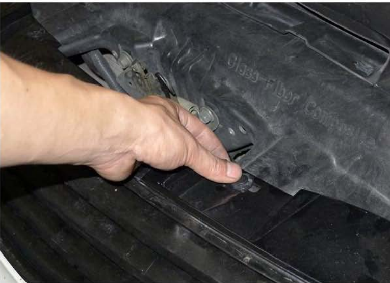
43. Replace the (6) plastic clips
