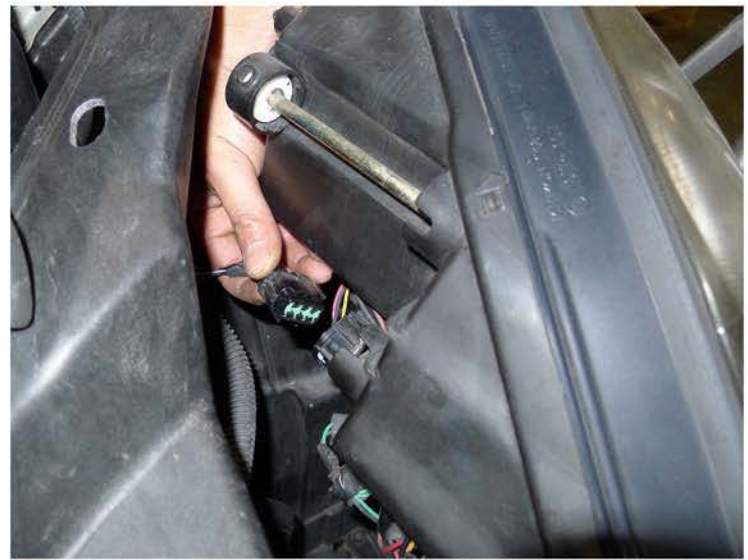
18. Disconnect the headlight harness
