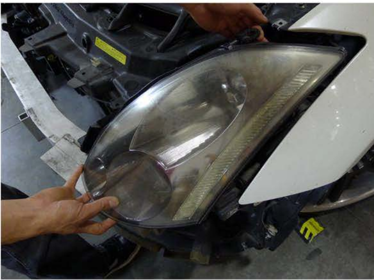
17. Remove the headlight
