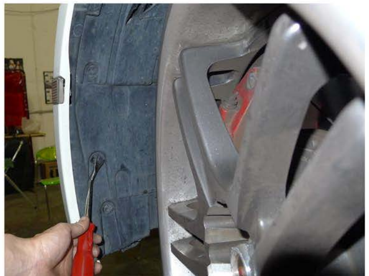
4. Remove the (3) plastic clips
