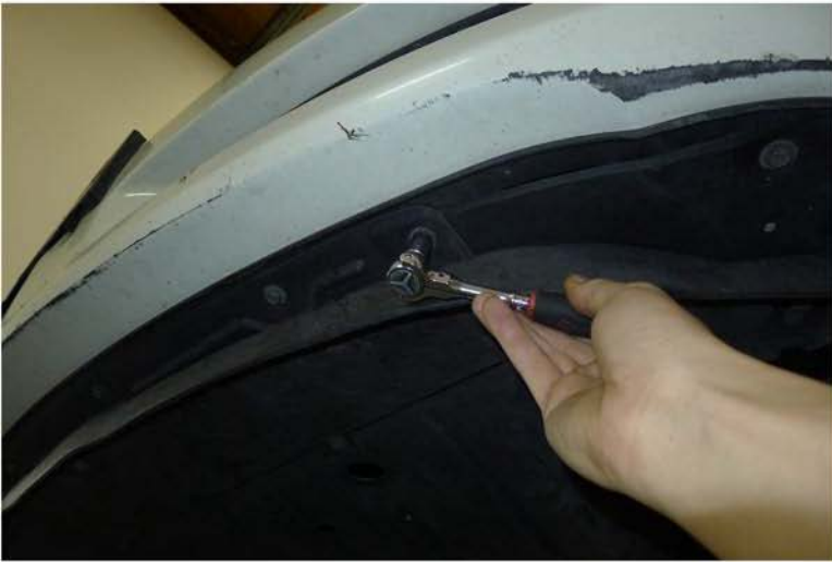
47. Tighten the (10) 10mm bolts
