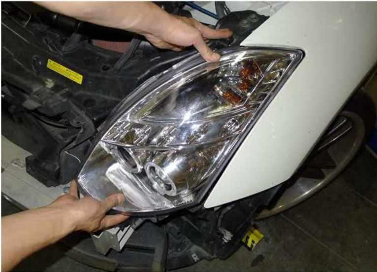
37. Place the new headlight in the stock location
