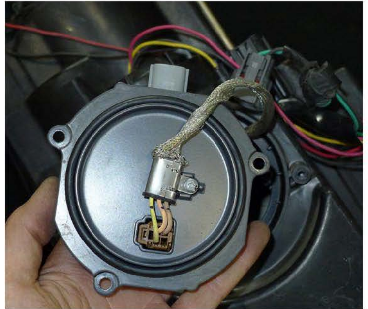
22. Back of the ballast
