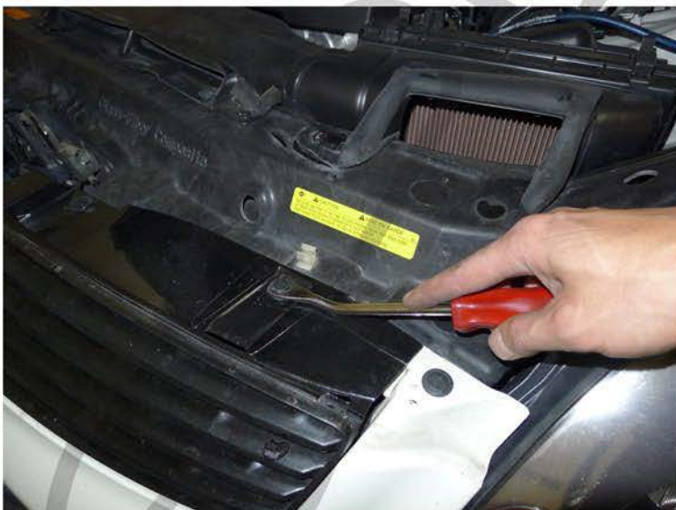
9. Remove the (6) plastic clips
