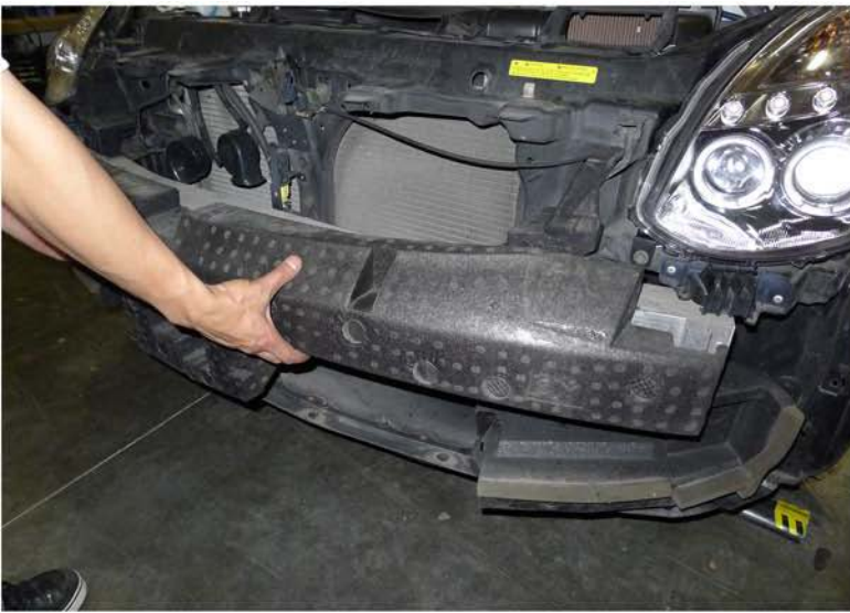
41. Replace the energy absorber
