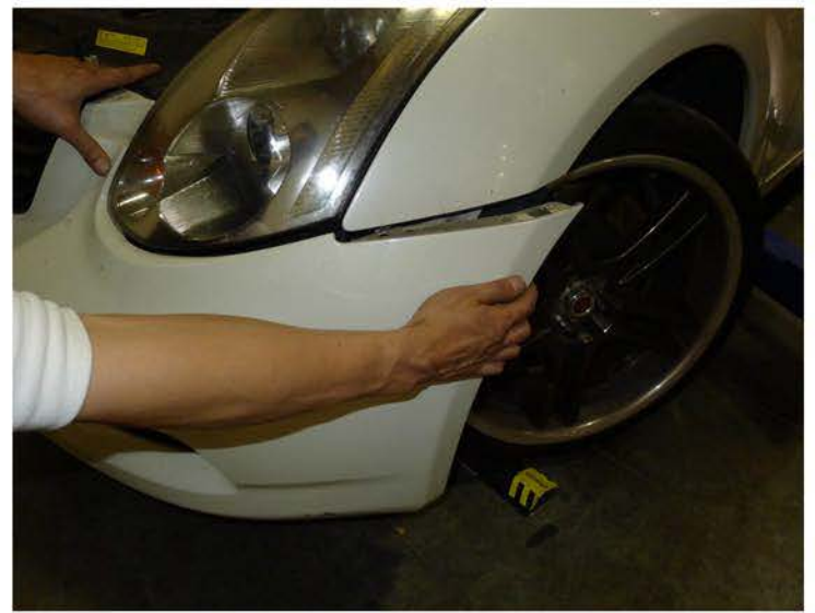
10. Pull the sides of the front bumper down and then outward
