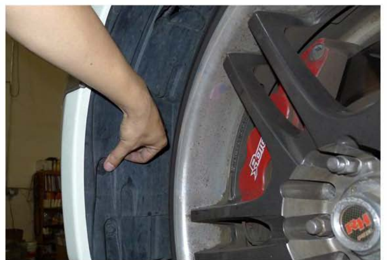
46. Tighten the (2) 10mm bolts
