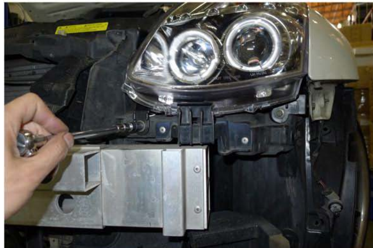
40. Tighten the (2) 10mm bolts
