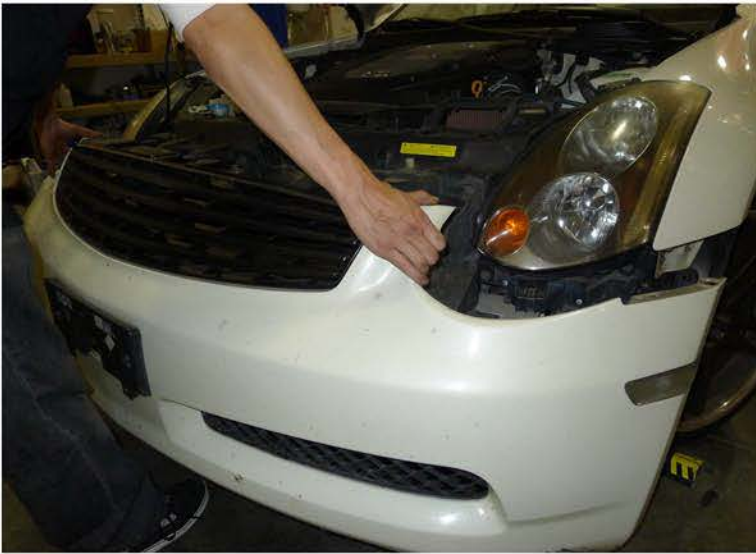
11. Remove the front bumper
