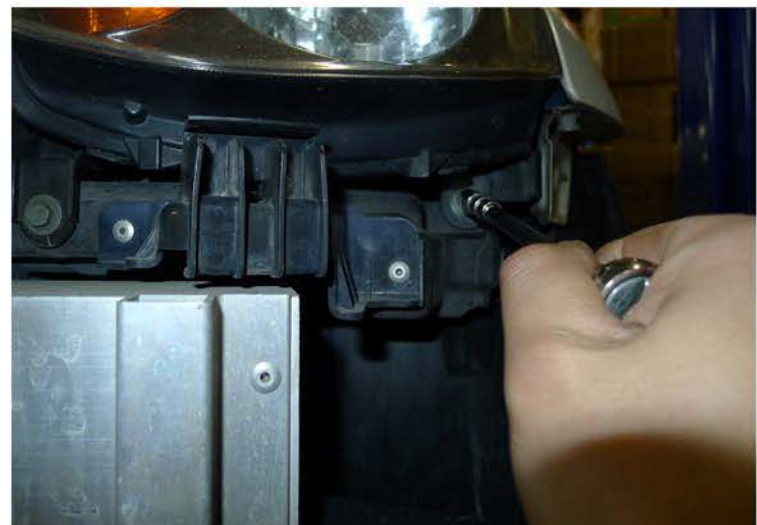
16. Remove the (2) 10mm bolts
