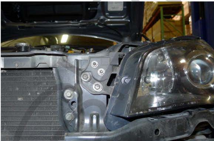
15. (2) 10mm nut and the (2) 10mm bolts location
