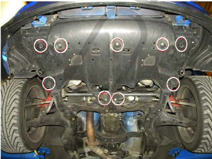
3. Remove five bolts and four clips
