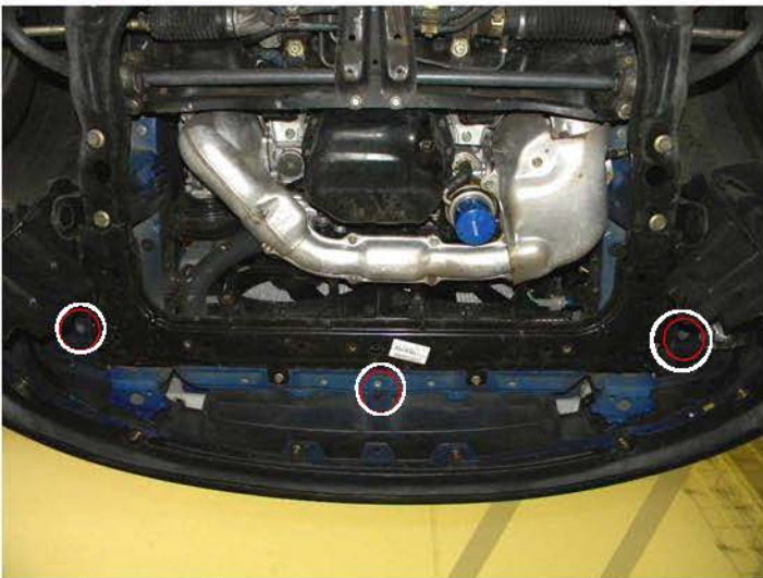
7. Remove three clips
