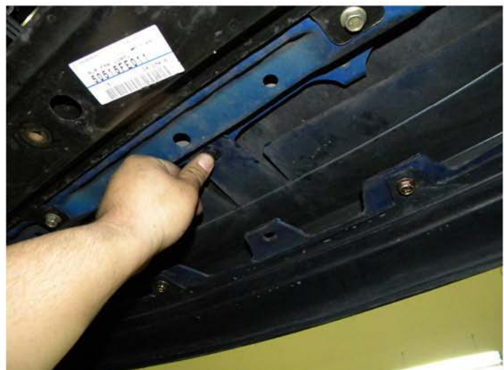
22. Install three clips
