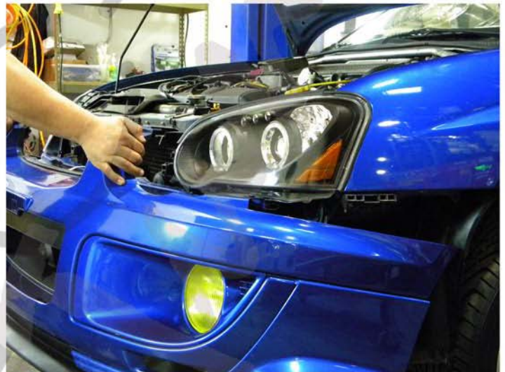
20. Install the front bumper
