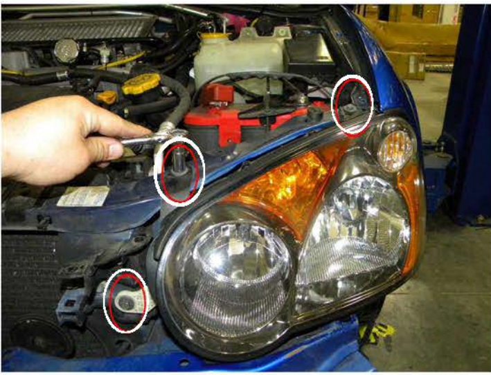
11. Remove three 10mm headlight bolts
