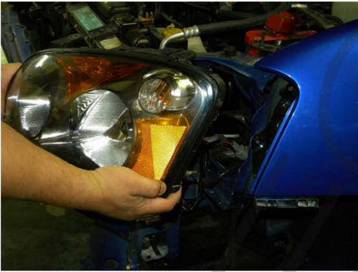
13. Remove the headlight
