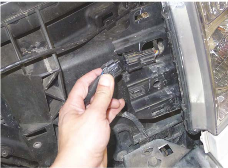
11. Disconnect the headlight harness
