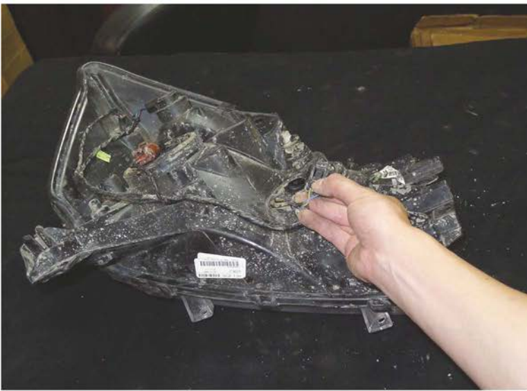
17. Remove the headlight sub-harness
