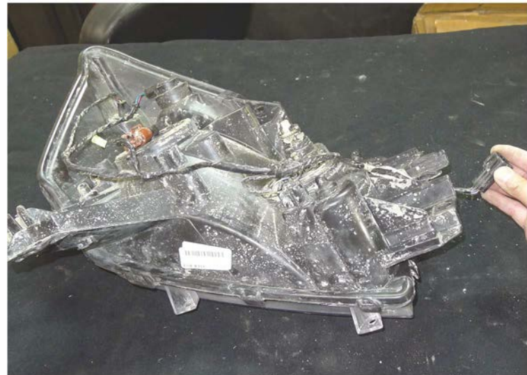
16. Remove the headlight sub-harness
