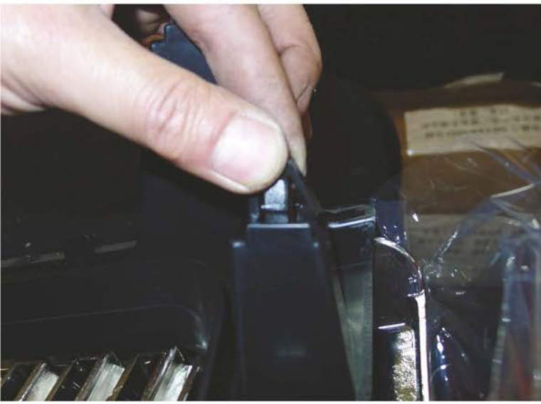
35. Install the plastic clips on the grill
