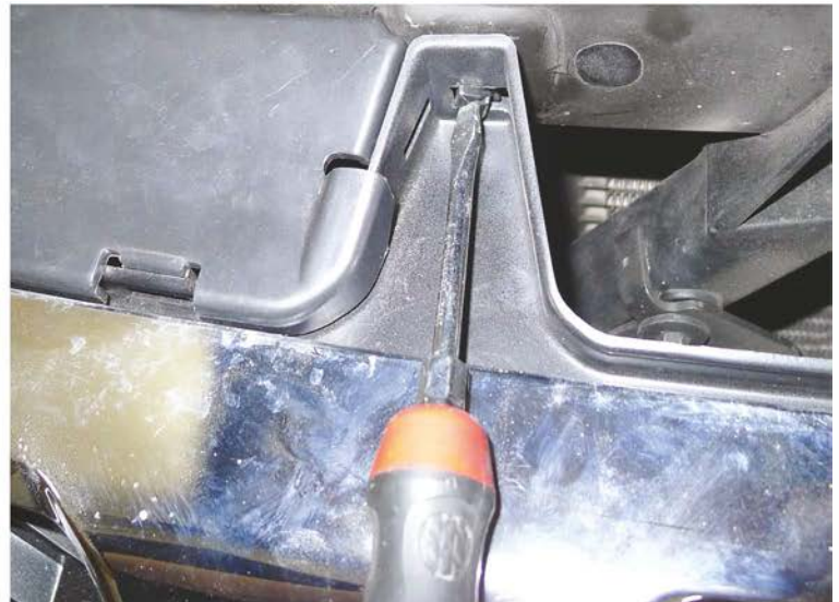
4. Release the plastic clips holding grill onto the radiator support
