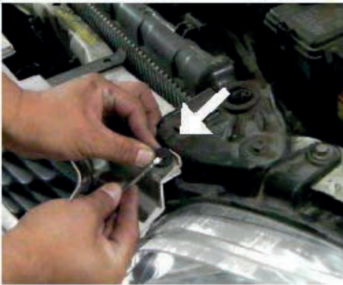
17. Install one clip for the front bumper
