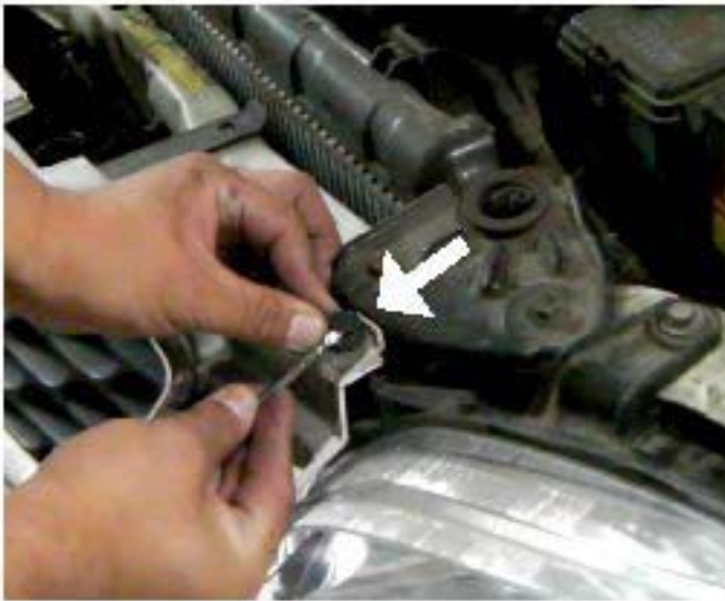
5. Remove one clip from the top of the front bumper
