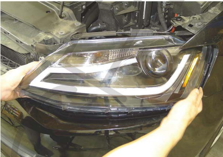
21. Place the new headlight in the stock location Please see the "Halo and L.E.D installation instructions"
