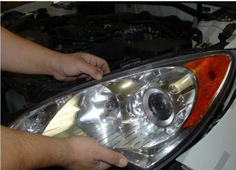
13. Remove the stock headlight and disconnect the headlight harness
