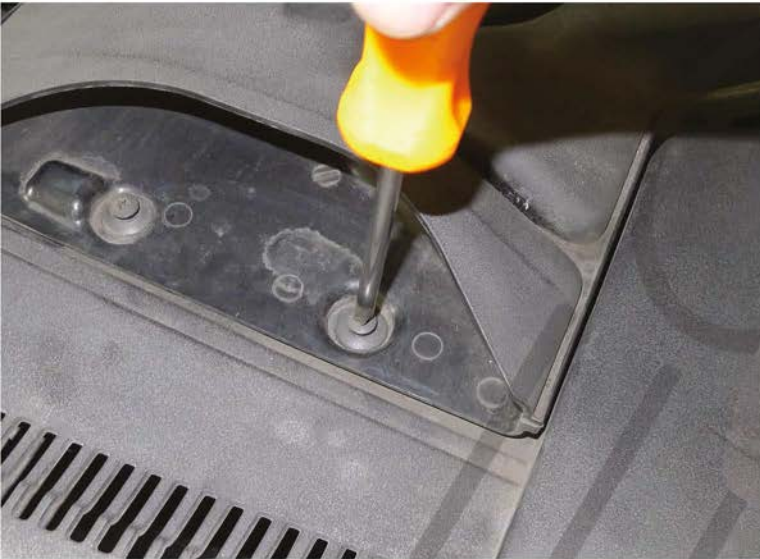
50. Replace the (2) plastic clips Please repeat the steps from 1 to 50 for the opposite side
