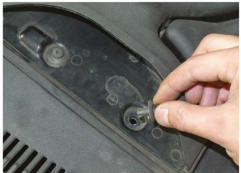
4. Remove the (2) plastic clips
