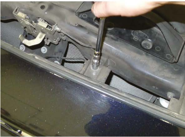
17. Remove the (5) 10mm bolts
