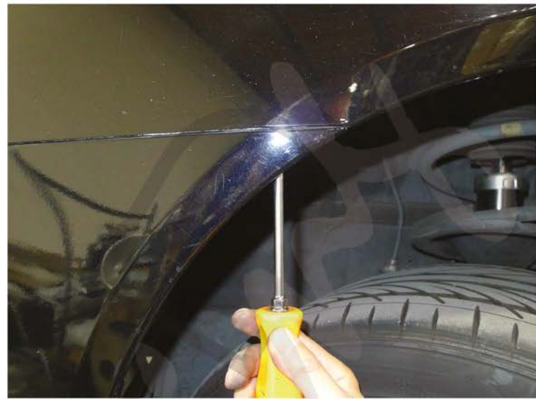
12. Remove the phillips head screw
