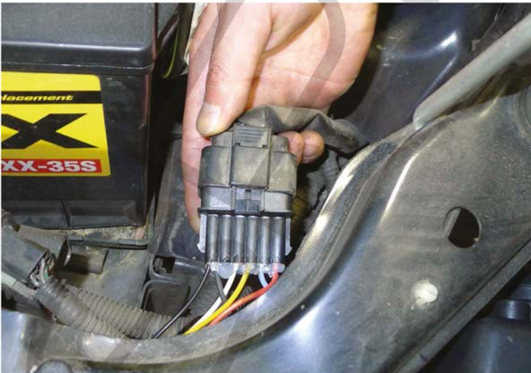
33. Connect the headlight harness to the projector headlight Please see the "L. E. D. head lights installation instructions"
