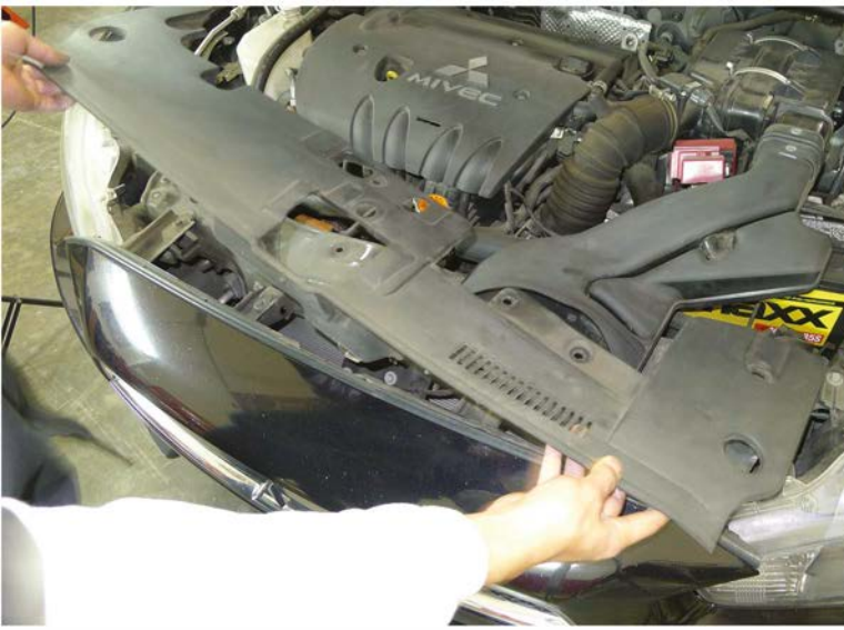
48. Replace the plastic moulding
