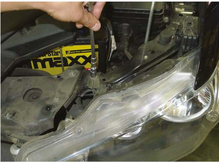
29. Remove the (3) 10mm bolts
