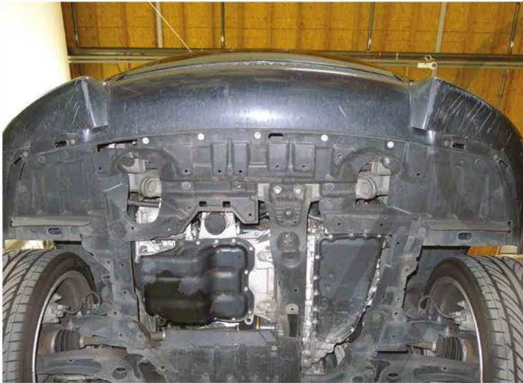
7. (6) plastic clips and the (5) 10mm bolts location
