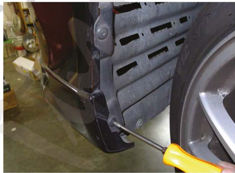
14. Remove the (2) plastic clips
