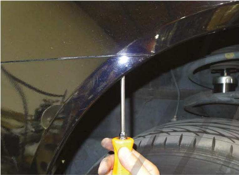
44. Tighten the phillips head screw
