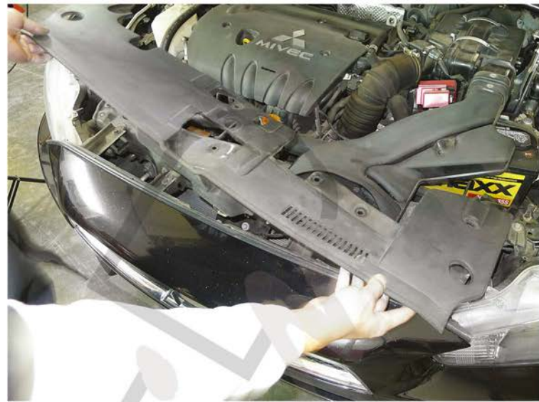
6. Remove the plastic moulding
