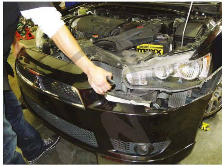
24. Remove the front bumper
