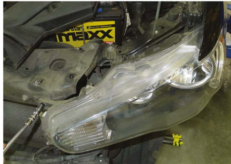
28. Remove the (3) 10mm bolts
