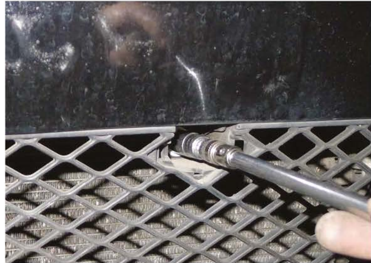
22. Remove the (2) 10mm bolts
