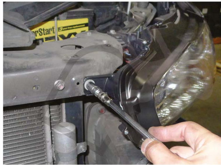
36. Tighten the (3) 10mm bolts
