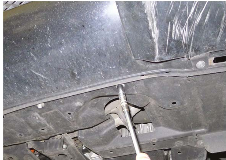
10. Remove the (5) 10mm bolts
