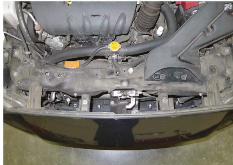
16. (5) 10mm bolts location
