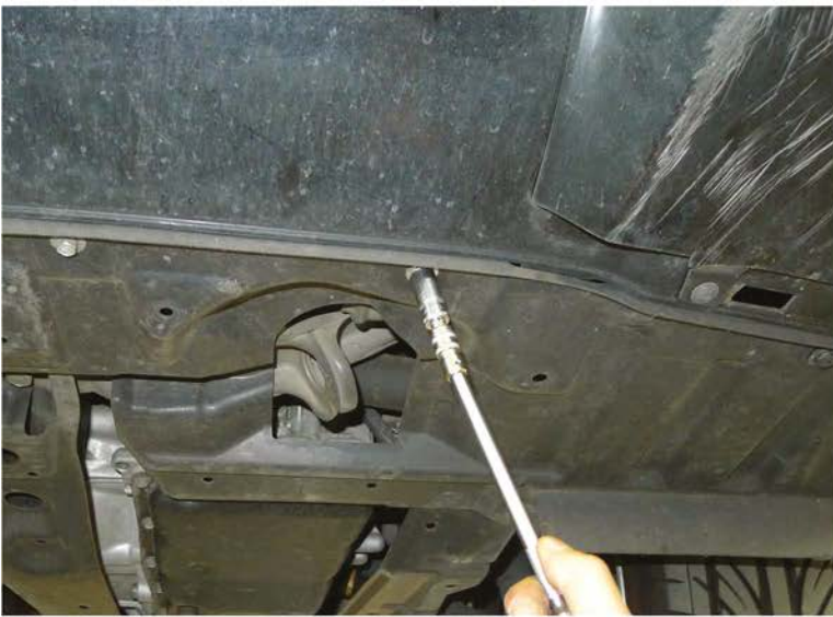
11. Remove the (5) 10mm bolts
