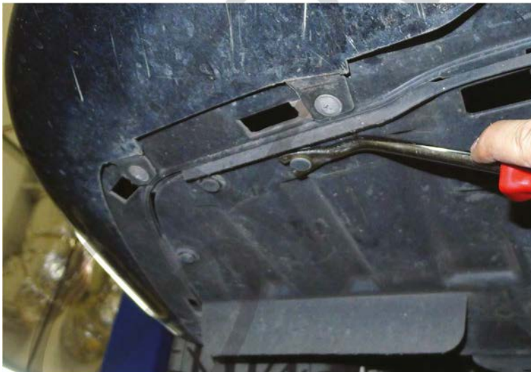
9. Remove the (6) plastic clips
