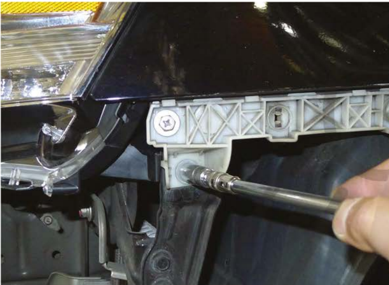
37. Tighten the 10mm bolt
