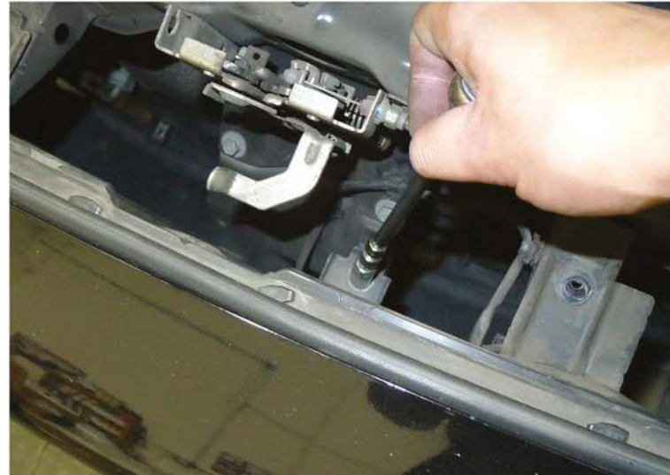
40. Tighten the (5) 10mm bolt
