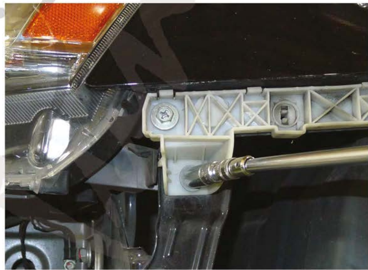
26. Remove the 10mm bolt
