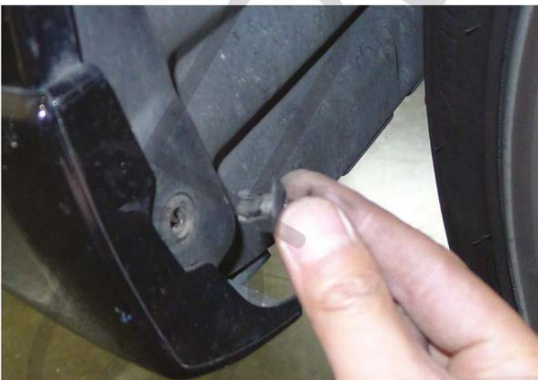
15. Remove the (2) plastic clips
