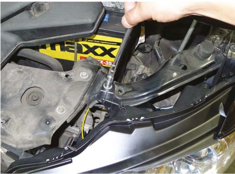
35. Tighten the (3) 10mm bolts
