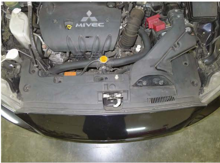
5. Remove the (4) plastic clips
