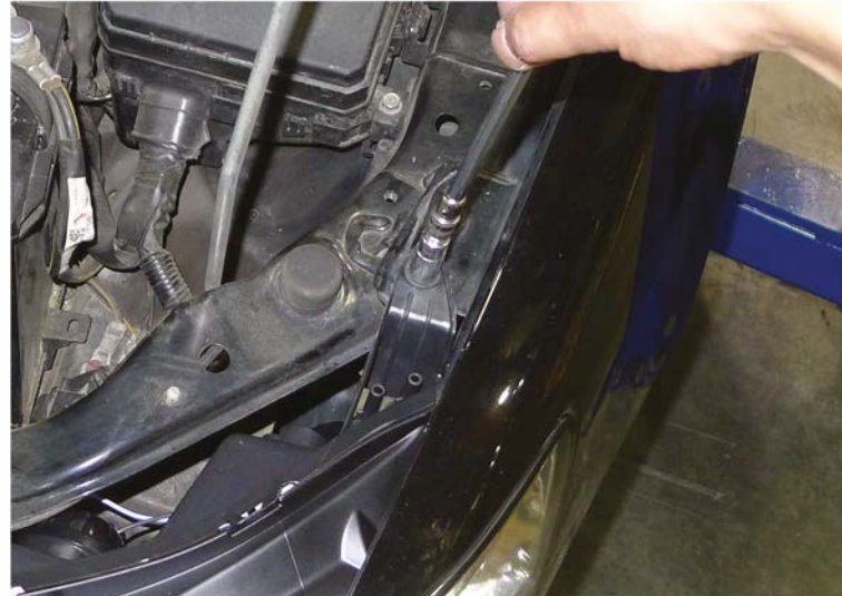
34. Tighten the (3) 10mm bolts
