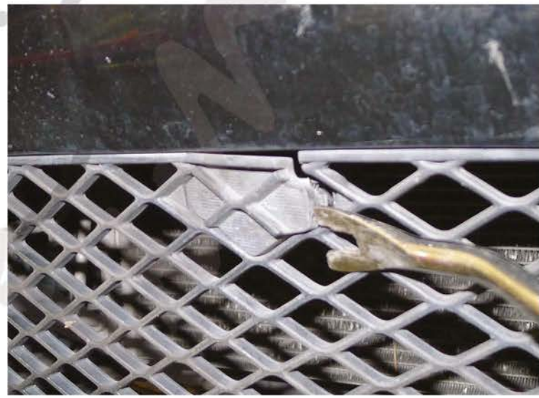
20. Remove the (2) plastic cover
