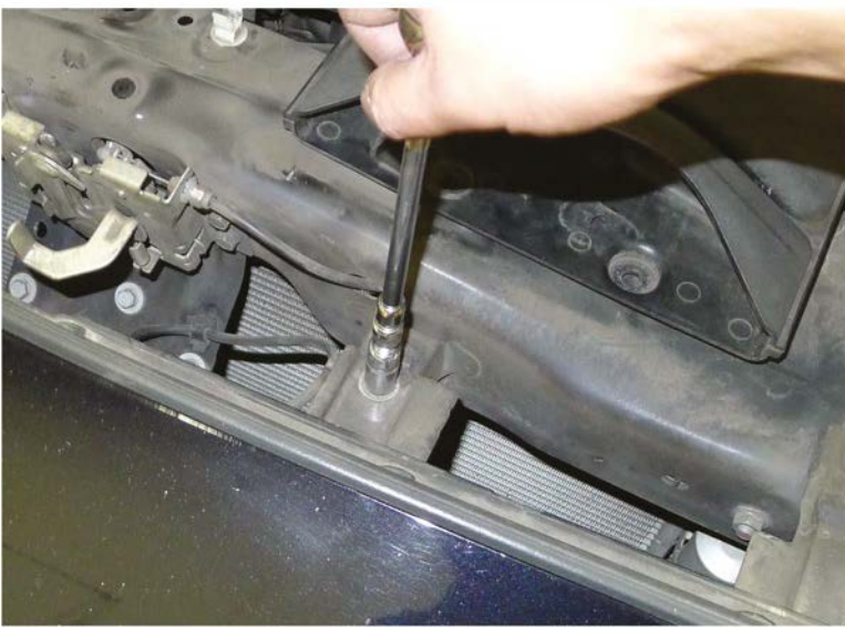
41. Tighten the (5) 10mm bolts
