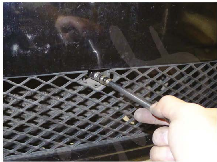
43. Tighten the (2) 10mm bolts
