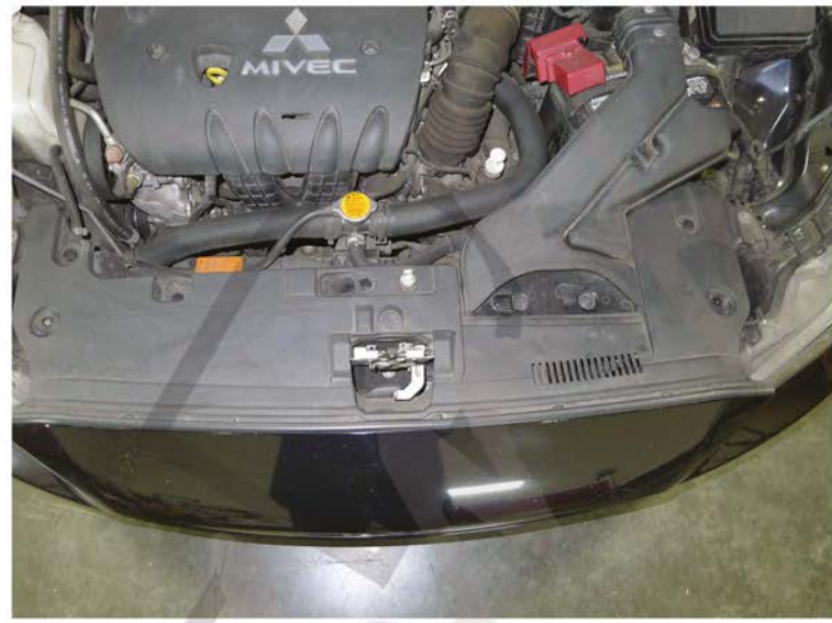
49. Replace the (4) plastic clips
