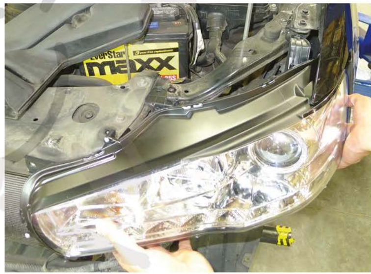
32. Place the projector headlight in the stock location
