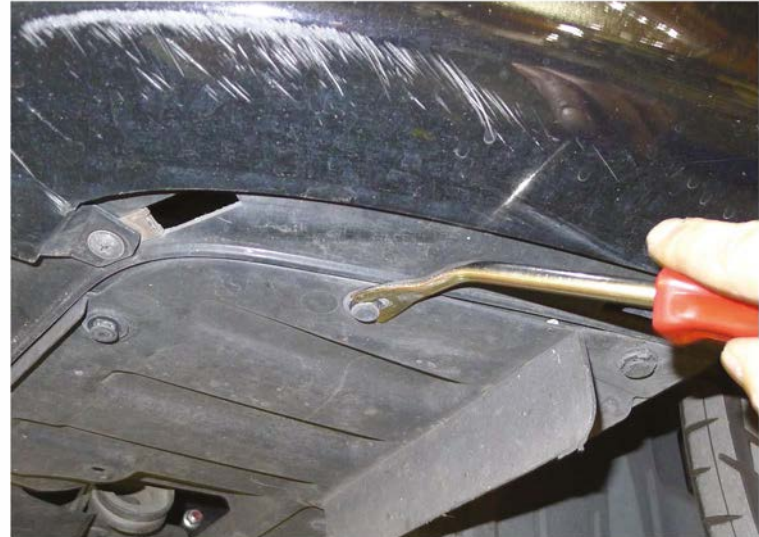
47. Replace the (6) plastic clips
