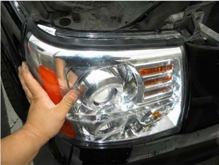
7. Install the new projector headlight
