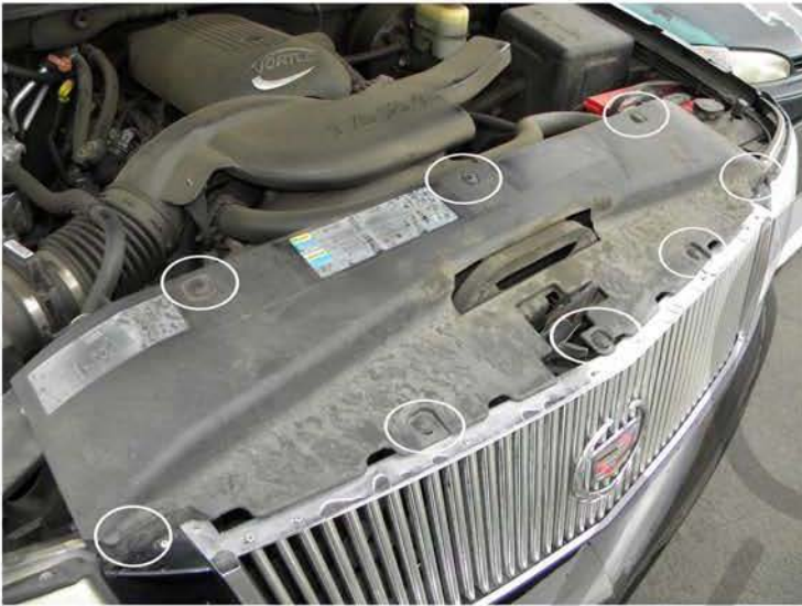
1. Remove the (8) clips then remove the plastic radiator cover
