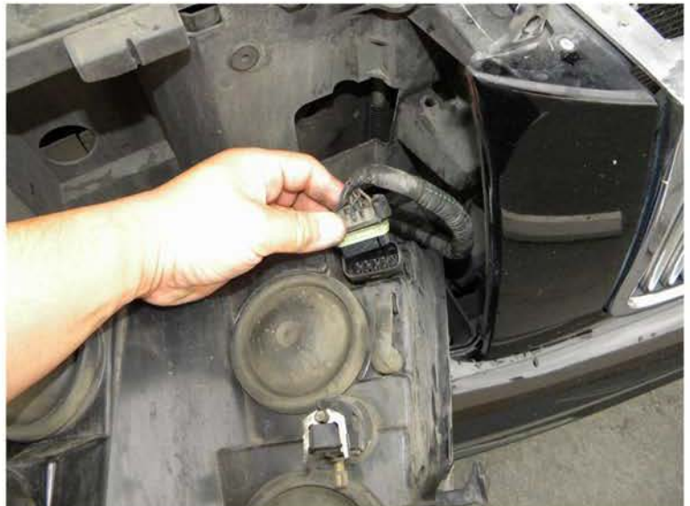
4. Disconnect the headlight harness
