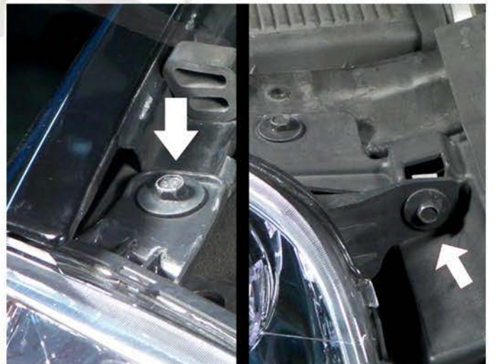
4. Remove two headlight bolts
