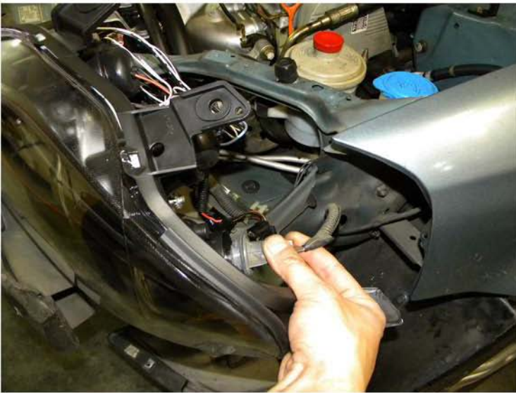
17. Plug in the light socket
