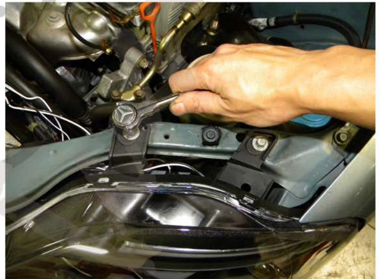
20. Tighten two 10mm bolts
