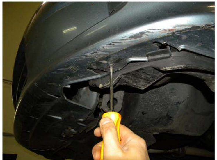
28. Screw in two phillips head screws under the front bumper
