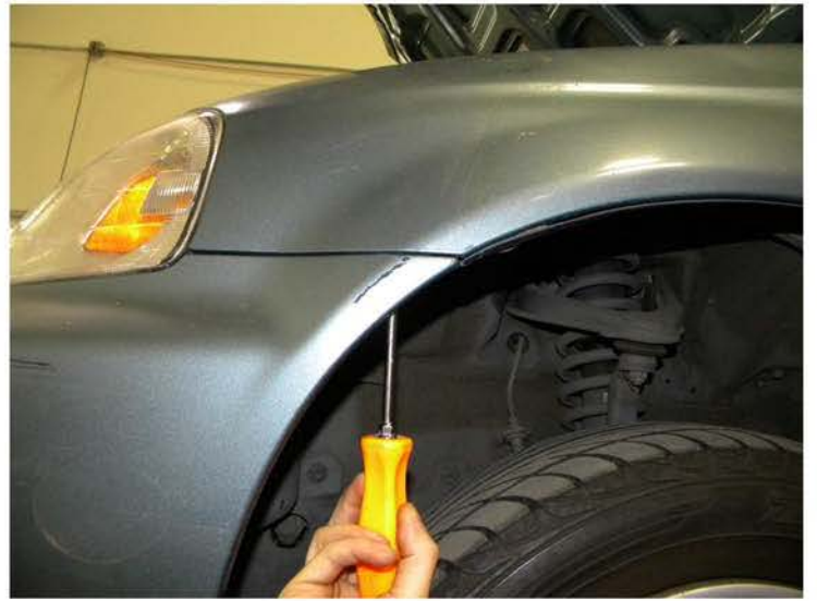
4. Unscrew a phillips head screw
