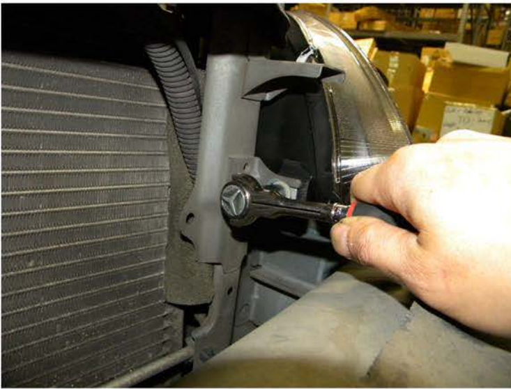
23. Tighten the 10mm bolt on the inner corner of the headlight
