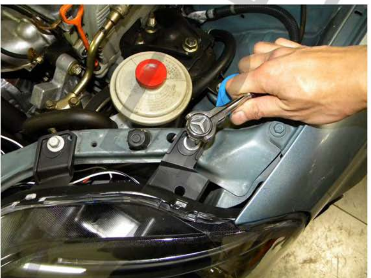
21. Tighten the second 10mm bolts
