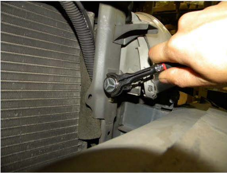
11. Remove the 10mm bolt on the inner end of the headlight
