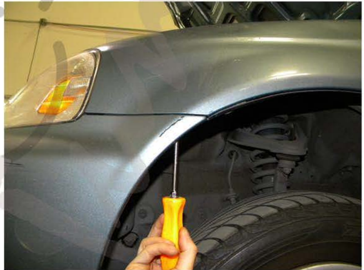
26. Screw in the phillips head screw
