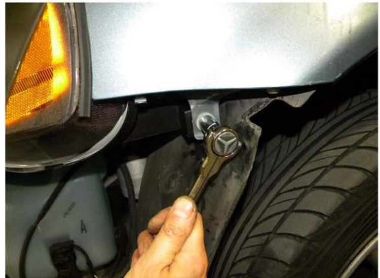
22. Tighten the 10mm bolt on the outer corner of headlight'
