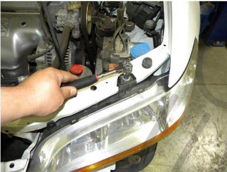
7. Remove one 10mm headlight bolt
