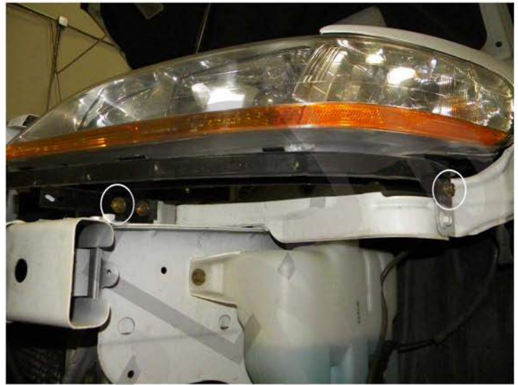
6. Remove three 10mm bolts, then remove the bracket
