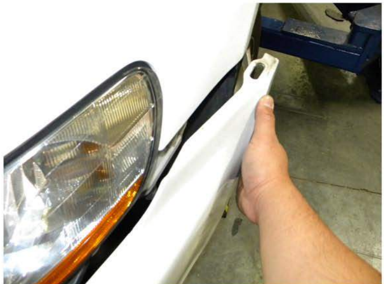
4. Pull out the front bumper from the side
