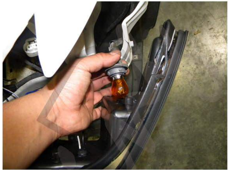
12. Plug back socket, install the new projector headlight
