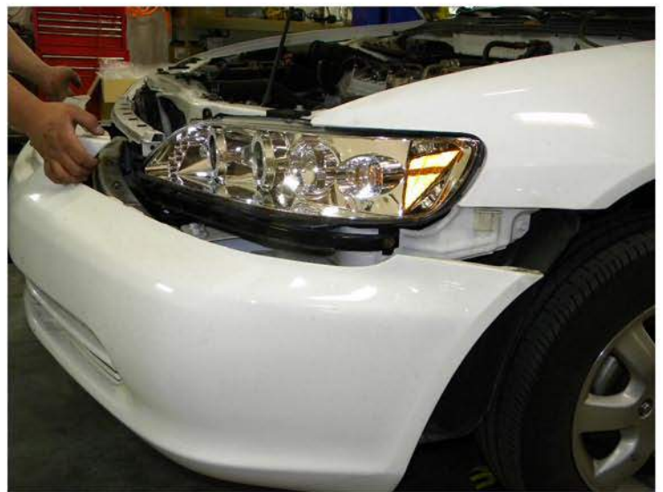
16. Install the front bumper
