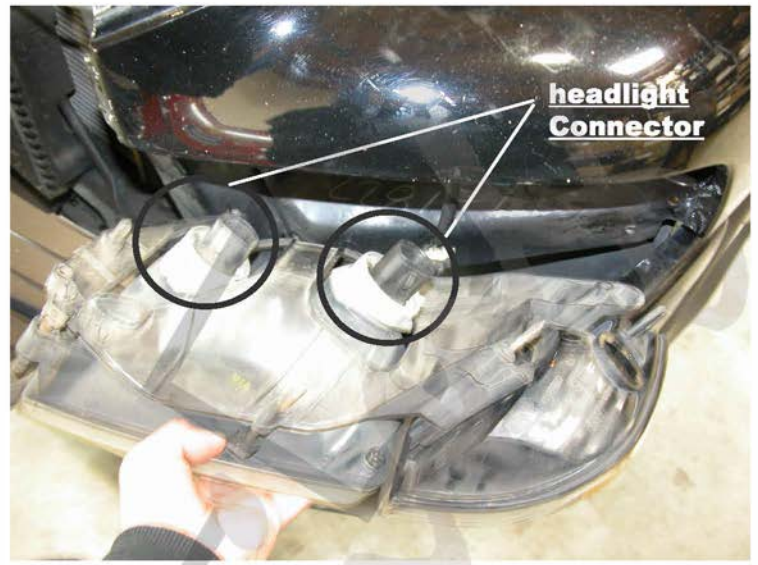
6. Disconnect the connector from headlight (BOTH SIDE)
