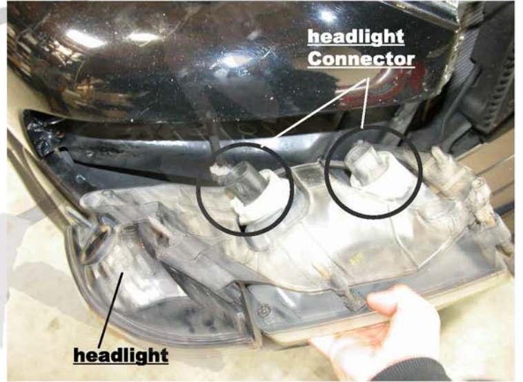
8. Connect the connector from headlight (BOTH SIDE)
