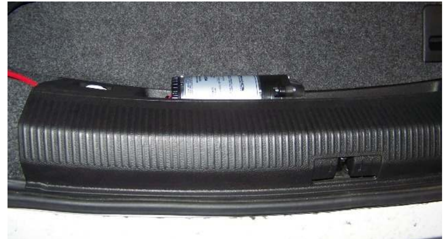
Pump Mounted below trunk opening.
