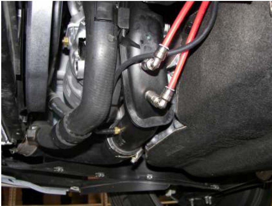
Nozzle mounted to charge pipe before EGR plate assembly. This view is from underneath the car, on the driver side.
