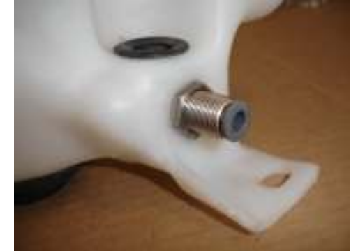
MKIV 5.5L Euro Spec Washer Reservoir VW PN 1J0 955 453 L & 2D0 955 465 B. Note that the bulkhead can be positioned on the side of the tank for easier tube routing to the pump.
