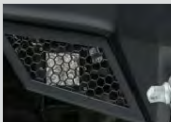
Removable mesh panels include provisions for 3"x3" LED cube lights
