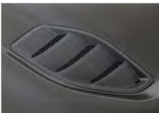
Vent hot gasses out of engine bay
