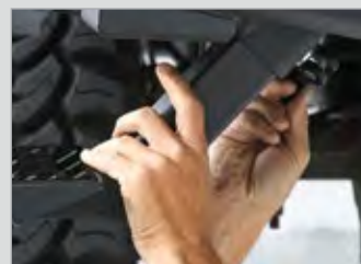
Adjustable rear steps have 4.7" of travel providing easy bed loading for any lift height
