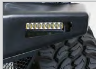
Front bumper includes 21" and (2) 6" LED light bars. Rear includes (2) 6" LED light bars
