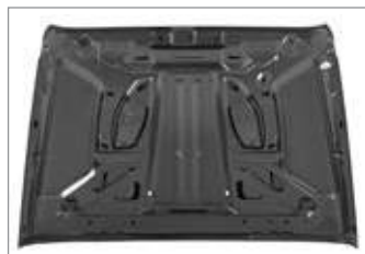
Factory crumple zones retained
