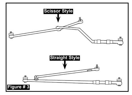
76-77 Ford F100 / F150 & Bronco. The drag link & tie rod assembly will require changing to the "Straight Style" steering in order to install a drop pitman arm. (See Figure # 3)
