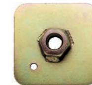
CCM10016 Eye-bolt back plate 65 mm x 65 mm x 3 mm 7/16" UNF thread welded nut, 40 mm 2 . Complies with FIA requirements.
