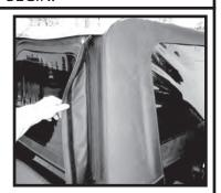
Step 2. Release the rear corners of the top. Pull down and out on the rear corners to remove the fabric from the belt rail. Repeat this procedures for both sides.
