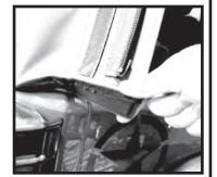
Step 3. Remove both sets of (4) Phillips head screws on the rear bow using a (#2) Phillips head screwdriver. Do not use power tools. Set the screws aside as they will be used to attach the new top.
