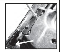
Step 9. With the assistance of a second person, raise the top and bow assembly in the up position. Lock the header to the windshield. With the top laying loosely over the bow assemblies, re-attach the fabric to the bows using the screws removed earlier. The fabric on the rear bow wraps under from the back side of the bow toward the front of the vehicle. The fabric on the middle bow wraps over the top and the front side of the bow.
