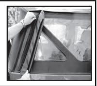
Step 13. Secure the top above the doors by inserting the plastic retainer strips into the door surround. Your new top installation is now complete.
