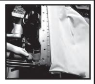
Step 7. Place the new top and onto the header with the bottom side of the top facing upward. With the top draped over the hood and windshield, locate the center notch on the top and the header. Once the two marks have been aligned, use tape to hold the top in position. Replace the top portion of the header over the soft top. Using the screws removed earlier, re-attach the top portion of the header.
