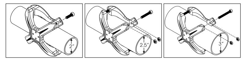
3. Select appropriate bolt length for your tube diameter. 2.5" and 3" diameter tubes require jam nuts. Note: to prevent jam nut interference with the high point of tube, keep jam nuts separate on bolt shaft during install.
