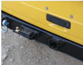
2" TOW RATED RECEIVER + SAFETY CHAIN HOOKS
