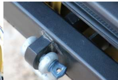
1" THICK STEEL DOUBLE WELDED RECOVERY TABS
