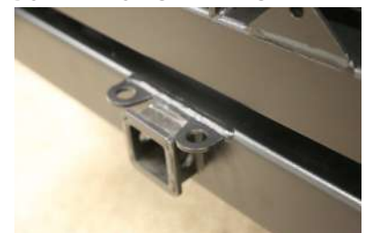
2" RECEIVER BUILT INTO BUMPER FOR CLEARANCE
