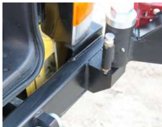
DROP DOWN SAFETY PIN PREVENTS CLOSURE
