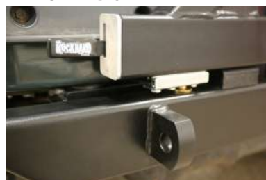
2 STAGE EASY TO OPEN LATCH AND STRIKER
