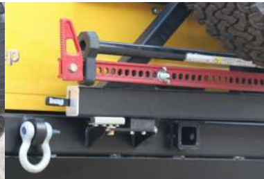
2 STAGE RATTLE FREE LATCH MECHANISM
