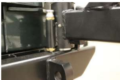
DROP DOWN SAFETY PIN PREVENTS CLOSURE
