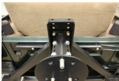
ADJUSTABLE SPARE TIRE MOUNT - FITS UP TO 38"
