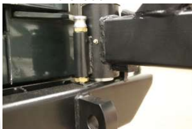
DROP DOWN SAFETY PIN PREVENTS CLOSURE
