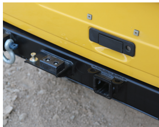
2" TOW RATED RECEIVER + SAFETY CHAIN HOOKS
