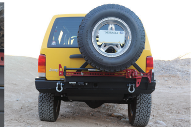
INTEGRATED HI-LIFT JACK AND CB ANTENNA MOUNTS
