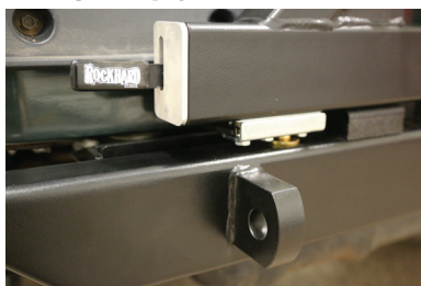
2 STAGE EASY TO OPEN LATCH AND STRIKER
