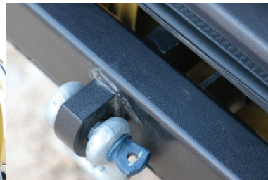
2 STAGE RATTLE FREE LATCH MECHANISM 1" THICK STEEL DOUBLE WELDED RECOVERY TABS
