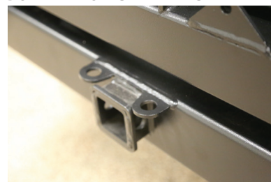
2" RECEIVER BUILT INTO BUMPER FOR CLEARANCE
