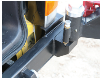
DROP DOWN SAFETY PIN PREVENTS CLOSURE
