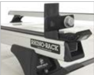
HI-LIFTING JACK HOLDER Mounts directly to Rhino-Rack Heavy Duty crossbar. Suits most hi-lifting jacks. Provision for pad lock. Use in conjunction with the Alloy Tray. PART NO: RJHB SUITS: Alloy Tray
